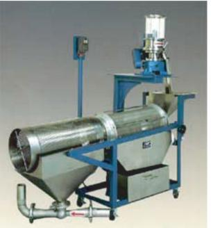
By adopting of a rotation type, generationg of the static electricity which is the risk of an oscillating type sorter was controlled. End powder is discarded without adhering to a pellet.
